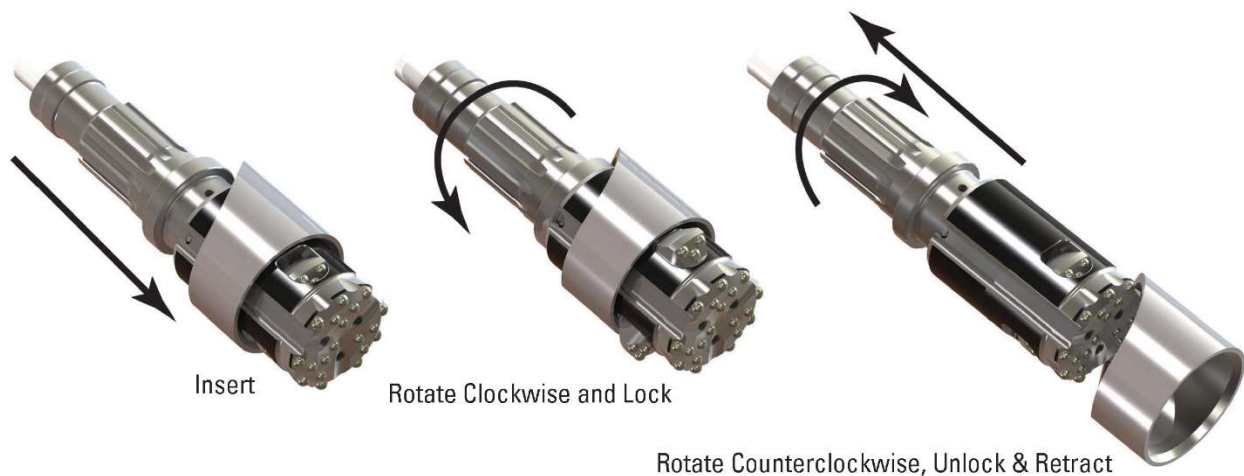
Figure 9. Expanded detail view demonstrating the operating principle of the Roto Loc under-reaming system manufactured by Center Rock, Inc.
